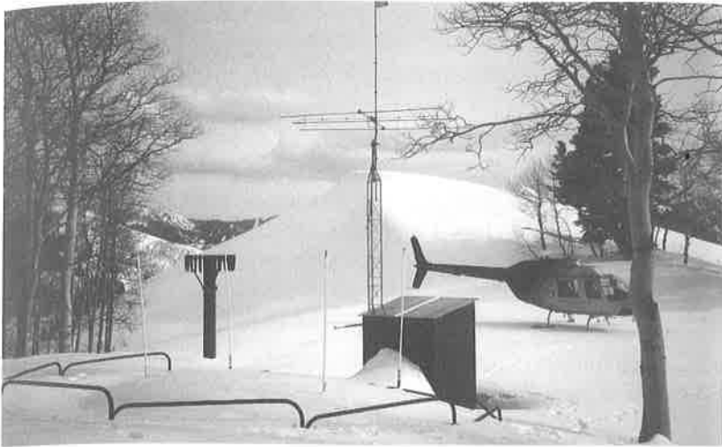
FIG. 2.8 Snow pillow station at a mountain station in Utah. An interesting website on snow pillow data, entitled “Seasonal Automatic Snow Pillow (ASP) Plots for B.C.,” can be found at http://www.env.gov.bc.ca/rfc/river_forecast/snowp.htm . The website is operated by the Water Stewardship Division of the Ministry of Environment, Government of British Columbia, Canada.
