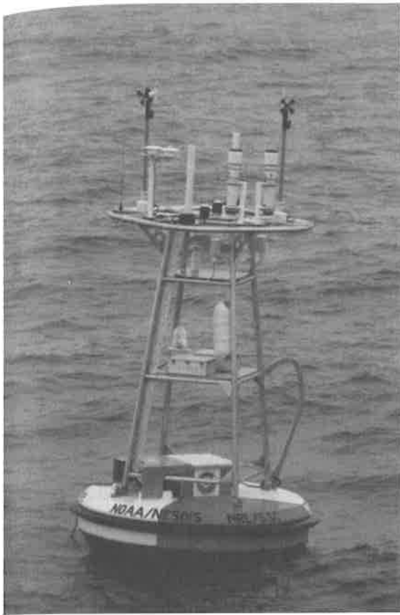
FIG. 2.21b Data are received by the National Data Buoy Center via a GOES satellite every three hours from buoys like this one. The information is used for improved ocean, weather, and climate forecasts.
