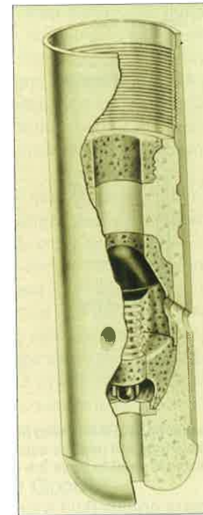
Figure 10.15. A cementing shoe has a ball-type check valve that prevents the grout from reentering the casing when the tremie pipe is withdrawn.
