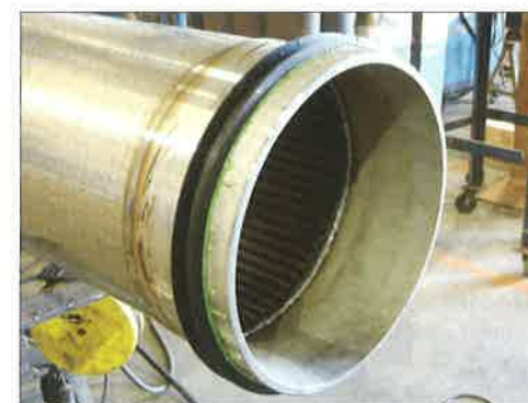
Figure 10.21. Self-sealing neoprene rubber packers (K-packers) form an effective seal between the casing and upper end of the screen or riser pipe.
