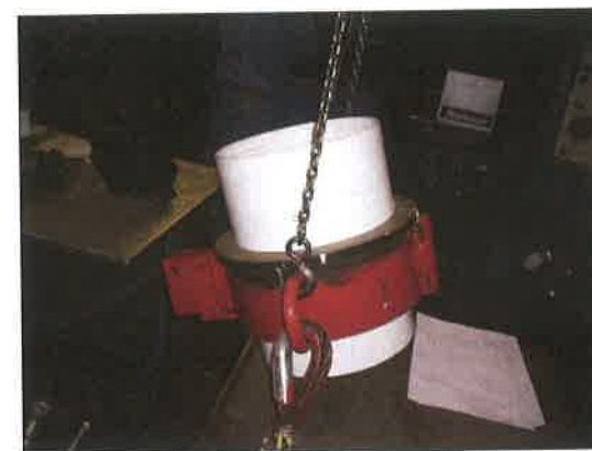
Figure 10.25. Elevator holding PVC pipe.
