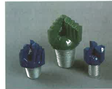
Figure 7.4. Drag bits are used in rotary drilling for fast penetration in unconsolidated or semi-consolidated sediments (Torquato Drilling Accessories).
