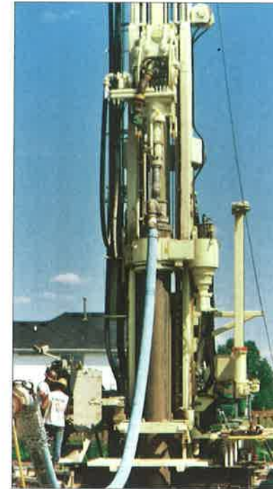
Figure 7.15. Casing rotator rig (Schramm, Inc.).
