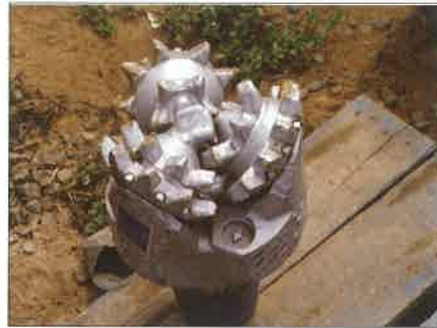
Figure 7.6. Roller-cone or other cone-type bits are preferable for drilling into consolidated rock.
