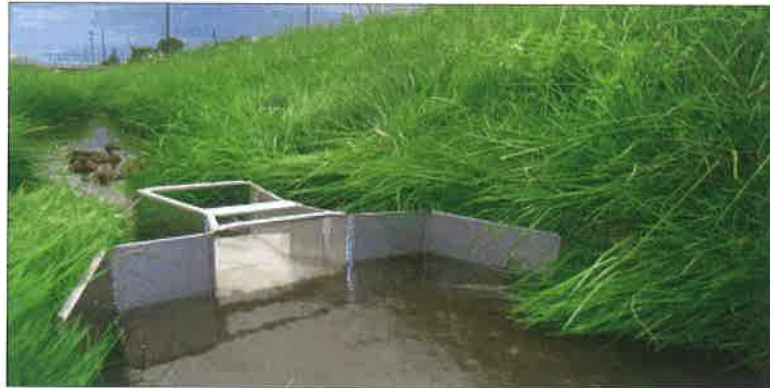
Figure 6.6. A collapsible cutthroat flume (Baski, Inc.).
