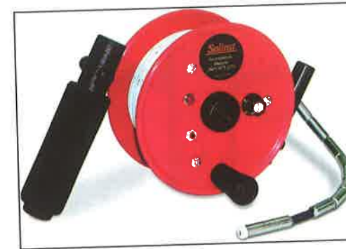
Figure 6.7. An electric sounder consists of an electrode, a two-wire cable, and a light which indicates a closed circuit when the electrode touches water (Solinst®).
