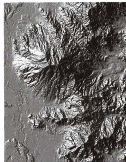
Figure 3. Bare earth/DTM rendition of LIDAR data of Mt. Tsukuba, Japan.
