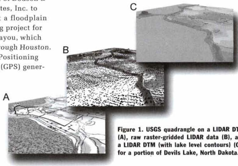
Figure 1. USGS quadrangle on a LIDAR DTM (A), raw raster-gridded LIDAR data (B), and a LIDAR DTM (with lake level contours) (C), for a portion of Devils Lake, North Dakota.
