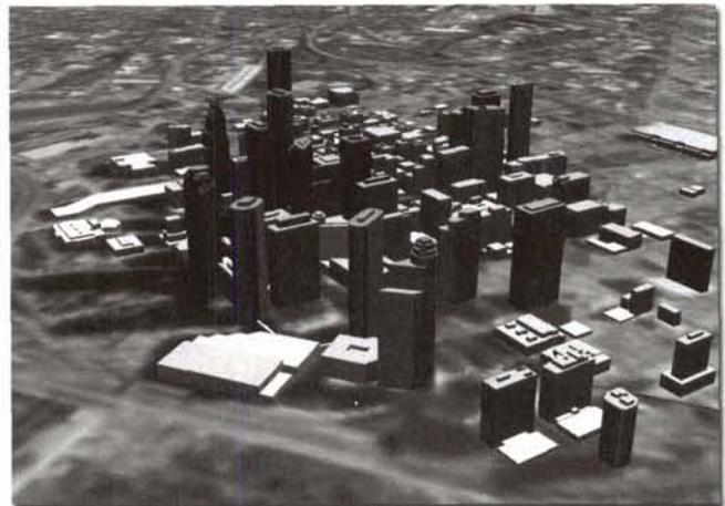
Figure 4. LIDAR-generated tall (above 10-meter) building rendition of downtown Houston, Texas draped on a USGS Digital Orthophoto Quadrangle (DOQ).
