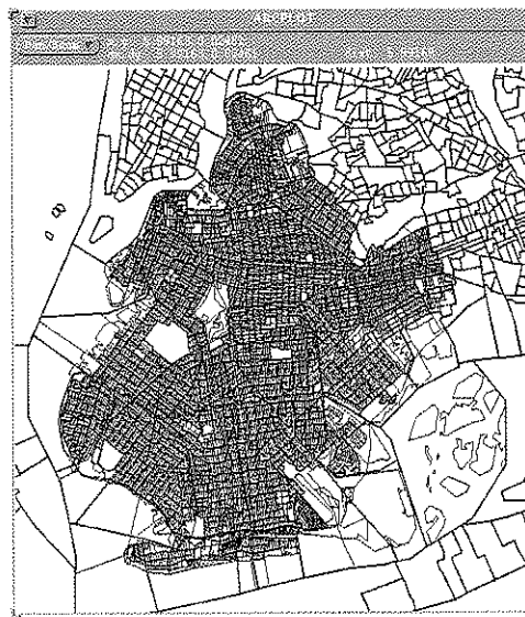
FIGURE 5.8: Map overlay. Example shows health districts and zip codes overlain for parts of New York city. The GIS can combine the two, so that attributes from one database can be cross referenced with the other. (Map by Barbara Tempalski.)
