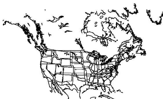
FIGURE 2.21: Mercator projection of North America secant at 40°N overlain with a Lambert conformal conic with standard parallels at 30°N and 45°N.
