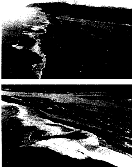
Figure 18. Rip currents cutting embayments through beach and reaching development on Siletz Spit during December 1972. Large embayment seen in upper photograph was center of property losses photographed in cover photo, lower right.
