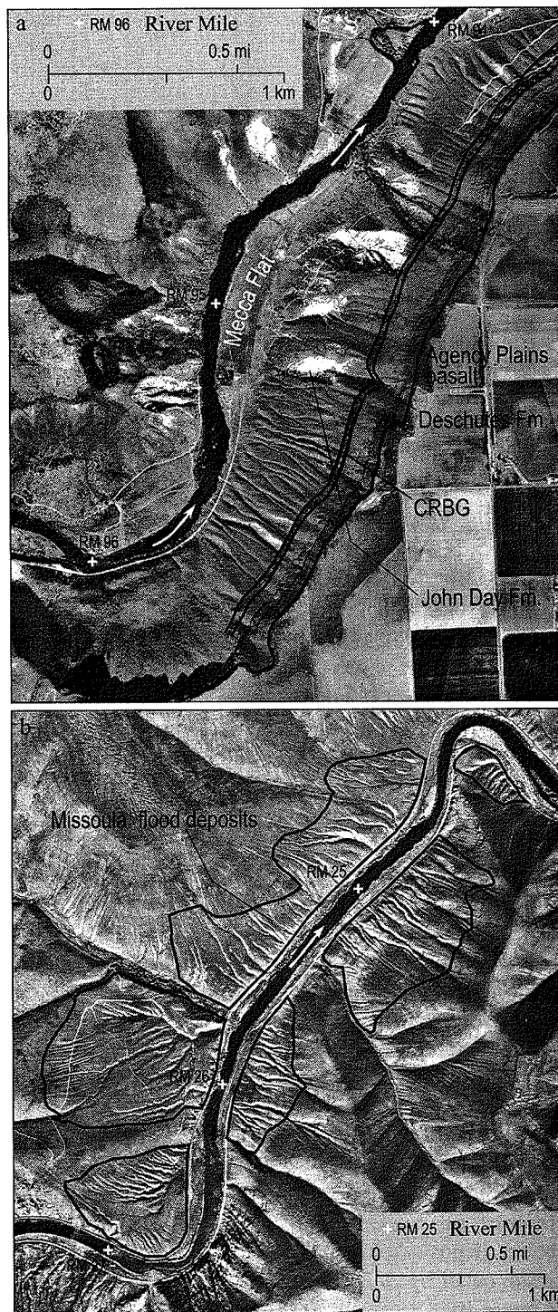
Figure 10. Vertical aerial photographs (1995, Portland General Electric) of gullies and rills. (a) Large gullies and rills in the John Day Formation near Mecca Flat at RM 95. CRBG is Columbia River Basalt Group. (b) Rills developed in Missoula flood sediment near RM 25. Missoula flood sediment mantles valley slopes developed in Columbia River Basalt Group.
