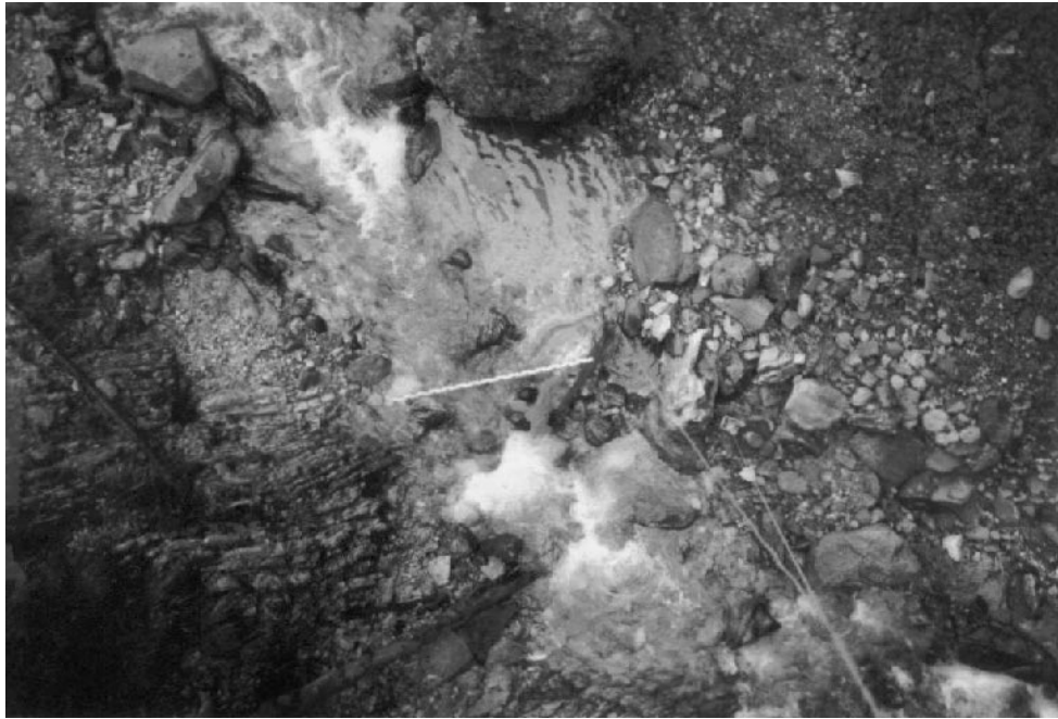
Fig. 4.14: Areal view of a step-pool reach at the Schmiedlaine, Bavaria (FRG) taken with a 35-mm camera mounted to a tethered helium balloon. Balloon height is about 15 m. Length of surveyor's rod is 3 m. Flow direction is from upper left to lower right. (Photograph courtesy of B. Kozłowski and P. Ergenzinger, Dept. of Physical Geography, Free University of Berlin, Germany).
