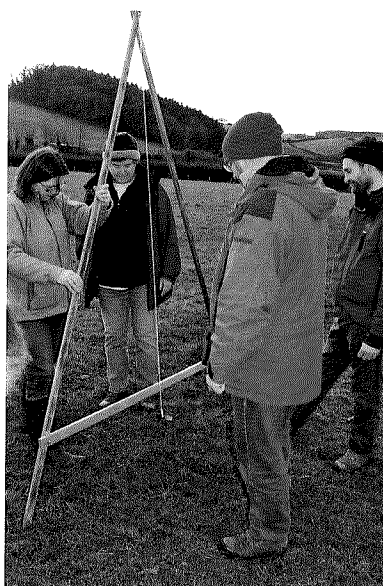
Marking out a contour using an A frame
