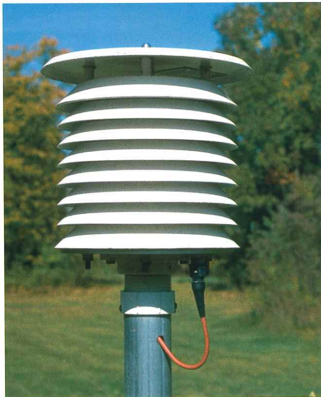
FIGURE 16.25 Measure Temperature This modern shelter contains an electronic thermometer called a thermistor . A shelter protects instruments from direct sunlight and allows for the free flow of air. (Photo by Bob Christopherson)
