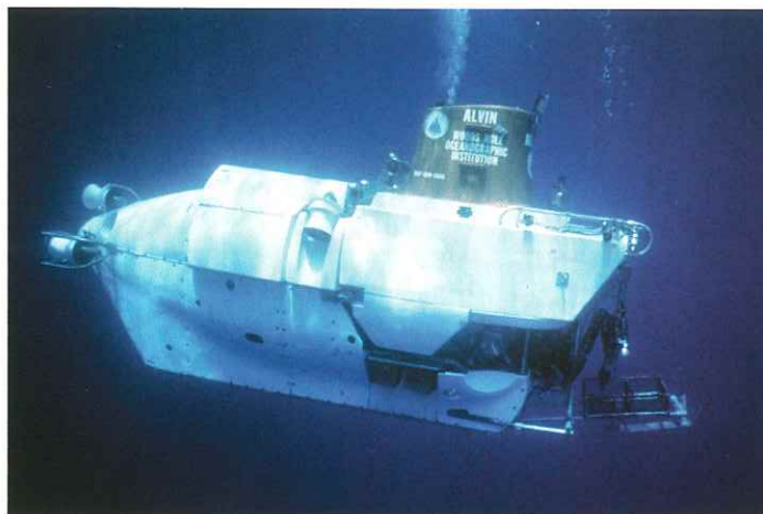
FIGURE 13.15 The Deep-Diving Submersible Alvin This submersible is 7.6 meters (25 feet) long, weighs 16 tons, has a cruising speed of 1 knot, and can reach depths of 4000 meters (more than 13,000 feet). A pilot and two scientific observers are along during a normal 6- to 10-hour dive. (Photo by Rod Catanach KRT/Newscom)
