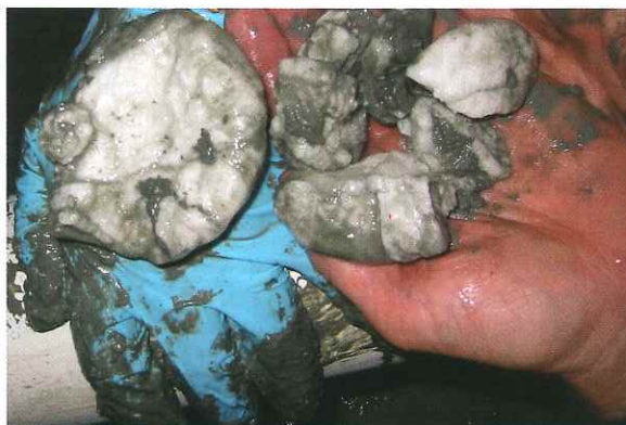
FIGURE 13.22 Gas Hydrates This sample was retrieved from the deep-ocean floor and shows white ice-like gas hydrate mixed with mud. Gas hydrates evaporate when exposed to surface conditions and release natural gas, which can be ignited. (Photo courtesy USGS National Center)
