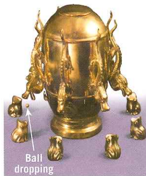
FIGURE 8.8 Ancient Chinese Seismograph During an Earth tremor, the dragons located in the direction of the main vibrations would drop a ball into the mouth of a frog below. (Photo by James E. Patterson Collection)
