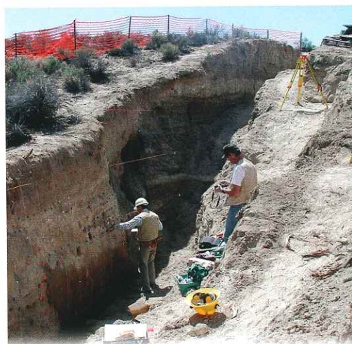
B. The events depicted in the accompanying diagram were deciphered by digging a trench (shown here) across the fault zone and studying the displaced sedimentary beds.
