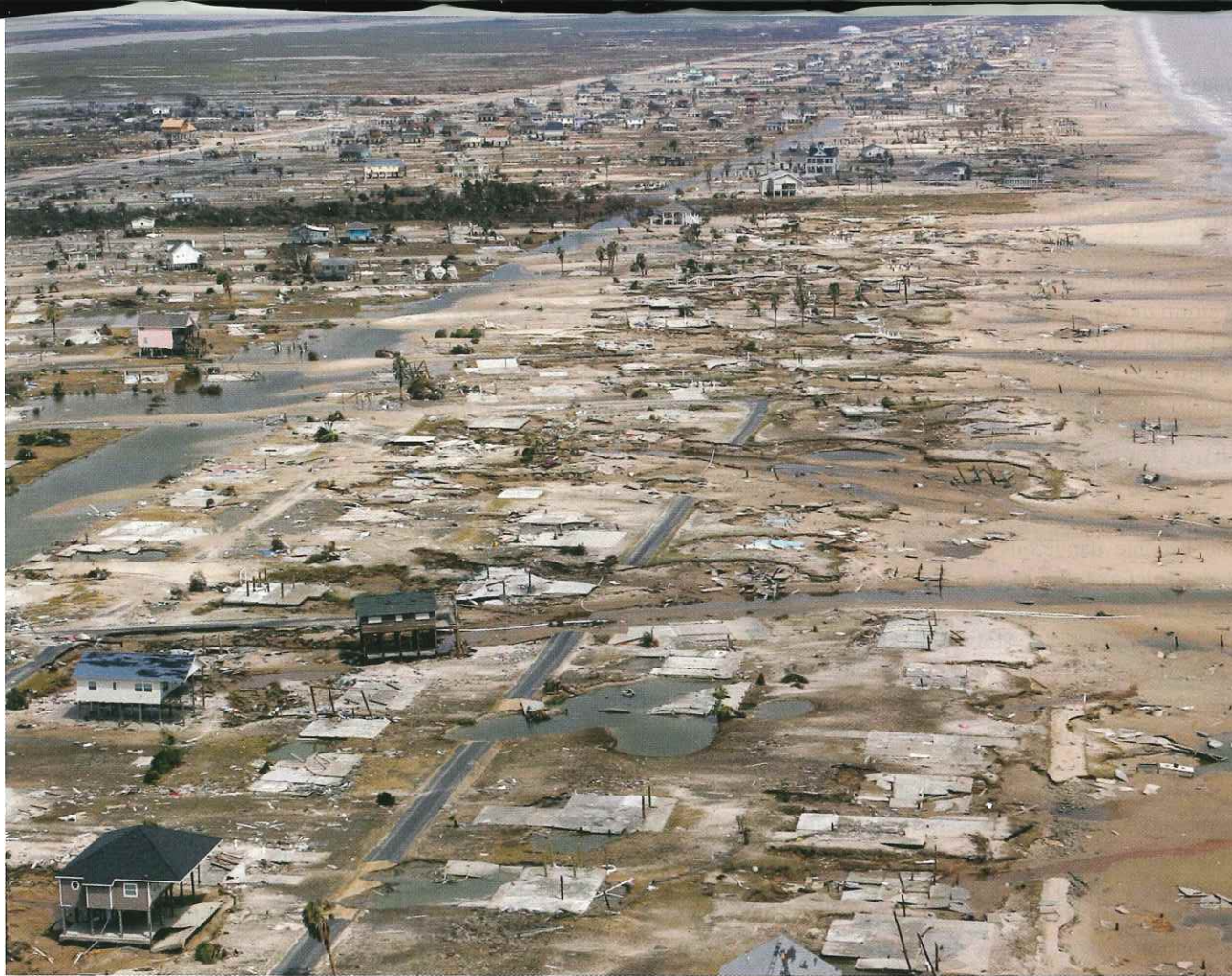
FIGURE 19.32 Storm Surge Destruction This is Crystal Beach, Texas, on September 16, 2008, 3 days after Hurricane Ike came ashore. At landfall the storm had sustained winds of 165 kilometers (105 miles) per hour. The extraordinary storm surge caused most of the damage shown here. (Photo by Texas Parks & Wildlife Dept., Earl Nottingham/AP Photo)
