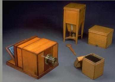
Right: the Giroux Daguerreotype camera, first mass-manufactured camera
