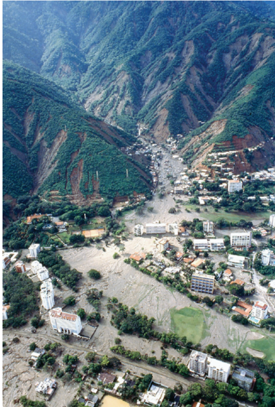
Fig. 1. Oblique aerial photograph of source areas and runoff paths of some of the devastating debris flows that were responsible for more than 20 000 fatalities in Vargas state, Venezuela, December 1999 (Photo by Matthew Larsen, US Geological Survey).
