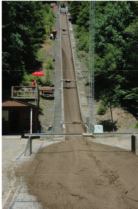
Fig. 4. Photograph of an 18 m 3 experimental debris flow discharging from the mouth of the 95-m-long USGS flume near Blue River, Oregon, USA (for details see Iverson et al. , 2010, 2011).
